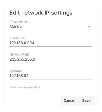
The gateway address is needed to access the internet when we connect LightStream Player to the router.
