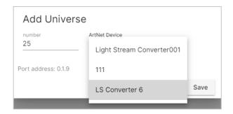
«Number» field indicates the number of the universe (numbering is end-to-end in accordance with the ArtNet v.4 protocol), additionally the number of the universe according to ArtNet v.3 protocol (Net.Subnet.Universe) is shown.
