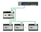
\* - If it becomes necessary to control the converters using Light Stream software, a PC with the appropriate network settings will need to be connected to the second port of the Converter, the last one in the chain.
