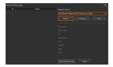
Select the network card in the «Ethernet Device» drop-down list, to which the converter is connected.
